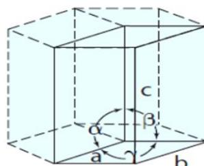
$$a = b \neq c \\ \alpha = \beta = 90^\circ, \gamma = 120^\circ$$
